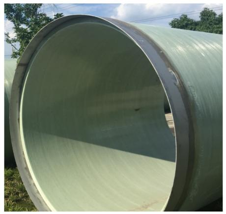
The production process of 12-meter-long fixed-length winding FRP sandwiched pipe is adopted, and four 3-meter-long FRP sections are produced on each mold at one time.
