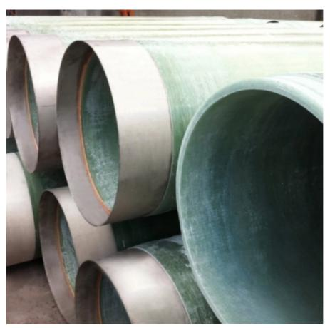
Embedded steel collar is used to connect and position the pipe segments, which is combined with fiberglass resin mouth sealing during jacking and water sealing after docking of the two pipes. The two ends of the jacking pipe are turned out on a
